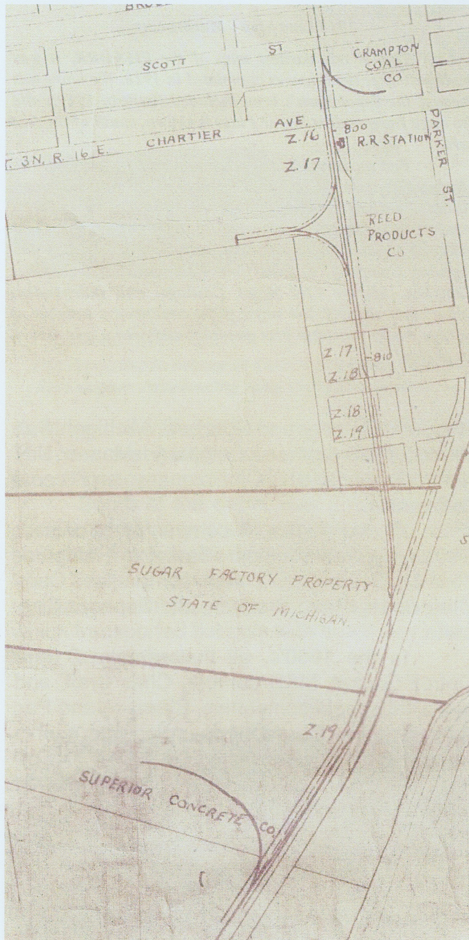
Superintendent William T. Frazier's Map of October 1959 shows the passing siding moved south of Chartier, no wye and the 19 mile mark. Note a small spur off the siding and a second Detroit Gasket Company spur. Our venerable M&D Lumber Company still exists.
