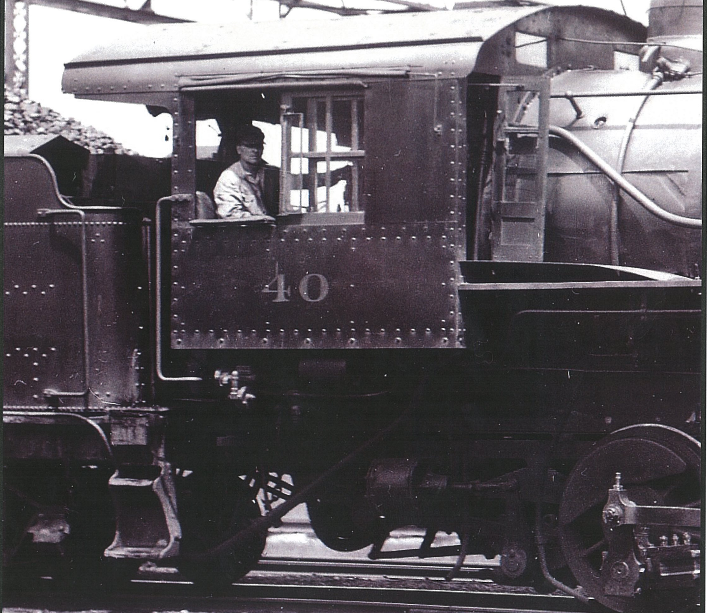
0-6-0 #40, Baldwin Class 6-38-D, at the 32nd Street yard. It would be retired in 1945.
