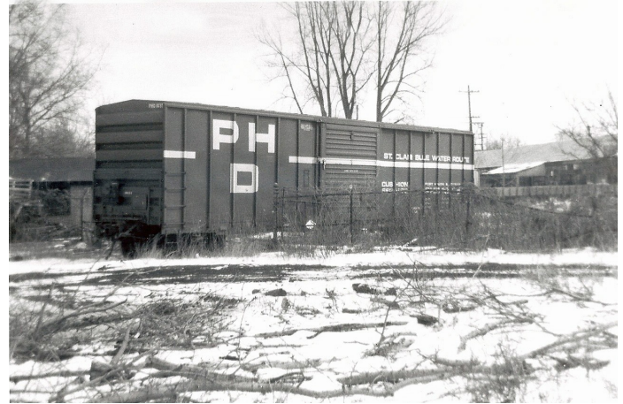
PH&D #1035 is at Pac-Lite, 1980. It was part of an order for 100 cars which arrived in the Spring of 1977. These cars were AAR designated "XM" loading for general purpose use. Photo: Don Cuthbertson Collection.
