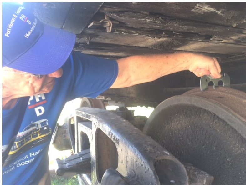
Former Roundhouse Foreman Bruce Sawdon measuring the flange on caboose #52. It would have passed.
