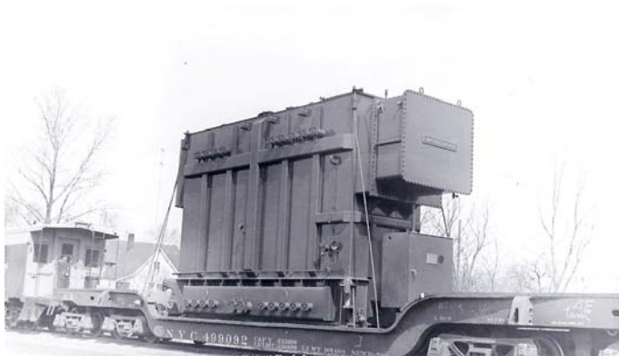
This generator was heading south, carried by a dropped center flat car with 16 axles and a capacity of 336,000 pounds. Wonder if this flat was ever produced in HO?
