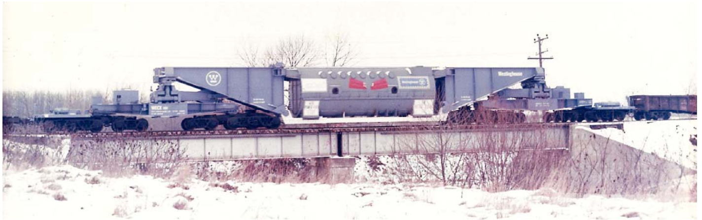
And here it is. They had to call in an old timer for this one. Prior to delivery, Superintendent Bill Munce had to make sure the line could handle a load weighing nearly 1,250,000 pounds. The biggest question was whether the old Pine River bridge, down in St. Clair, could withstand the weight. They called the one man who knew: the man who built the bridge back in 1926, retired Chief Engineer Bill Boyd. Here he was, a Snover farm boy, amidst top executives from the Detroit Edison, assuring them it could be done. “Old school” mathematics.
