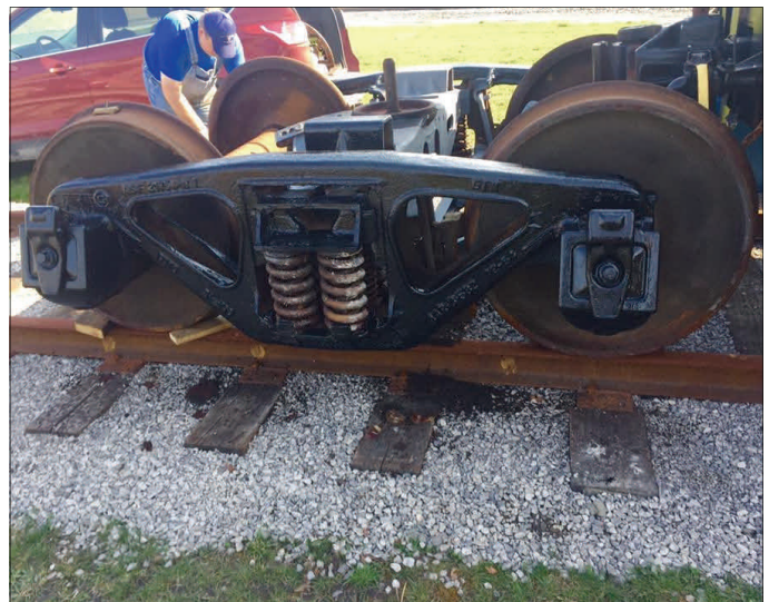
After being primed, a coat of protective industrial-strength black paint applied on one side. The second set of trucks will be delivered shortly.
