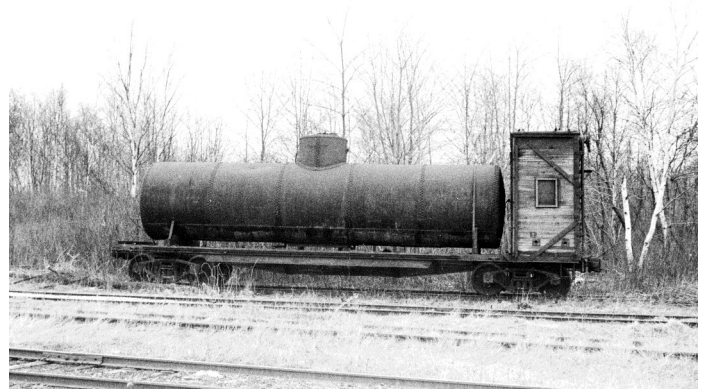
Charles included the weed sprayer, converted from an outside braced wooden boxcar that had been in an accident down at the Diamond Crystal Salt Co. A modelling project?
