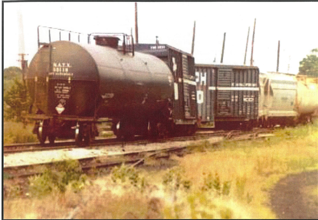
Trouble. Looks like someone's split the switch! NATX 35118 remains between the rails unlike the two ribbed side PH&D cars. The tank car is close to our 1974 date range (33800-35008) in this photograph taken 6-8 years later.
