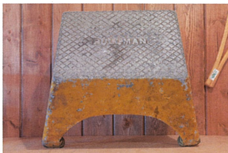
Many companies produced the Pullman step box and all adhered to strict design standards. All had the raised diamond pattern with "Pullman" in the center.
