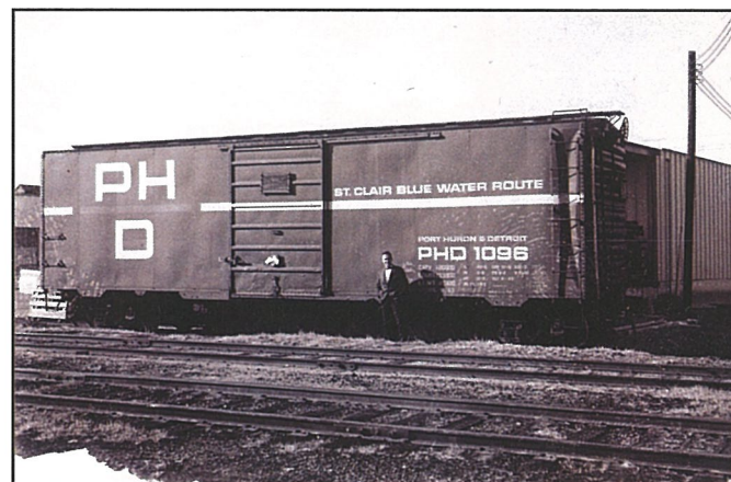
First series (1001-1277), 277 cars. Inside height 10'. Vice-President of sales Frederick Soini stands in front, called to the Chrysler receiving dock to investigate the damage beneath the ladder. Build date is "4/48". Rebuilt 1962. (photo: Duffy Collection)
